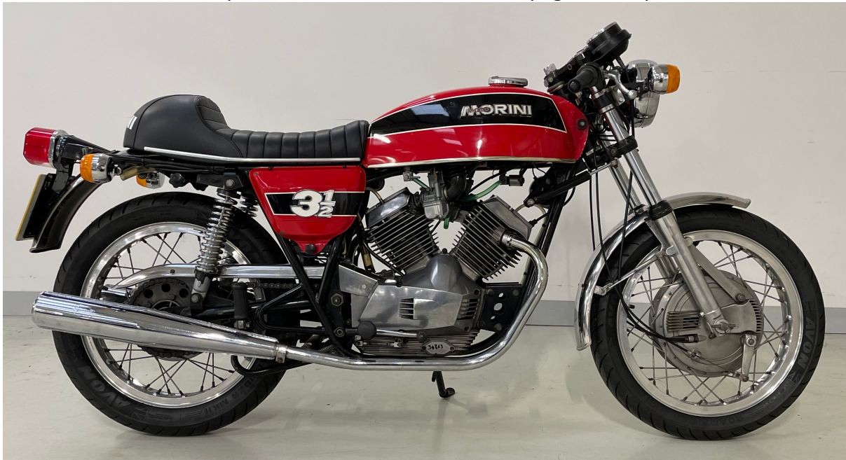
1975 Morini 350 sport. Electric fuel tap can be seen under the tank, with the green fuel hose connected to it
